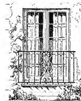
WROUGHT IRON RAILING
