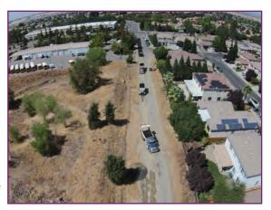
converted the 36-inch-diameter force main to a gravity trunk line. The project brought more than 5,000 feet of sewer trunk line into service, eliminating the need for two pumping stations and miles of force main. Installation methods and special techniques included dewatering; deep shoring and CLSM backfill for the sewer trunk line; construction of
